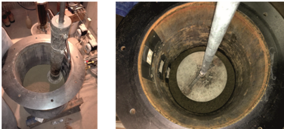
Fig. 16: Tools for material compaction
