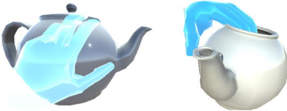
Figure 3.19: Left: Semi-transparent hand mesh rendered before contact. Right: Opaque hand mesh rendered during contact.
