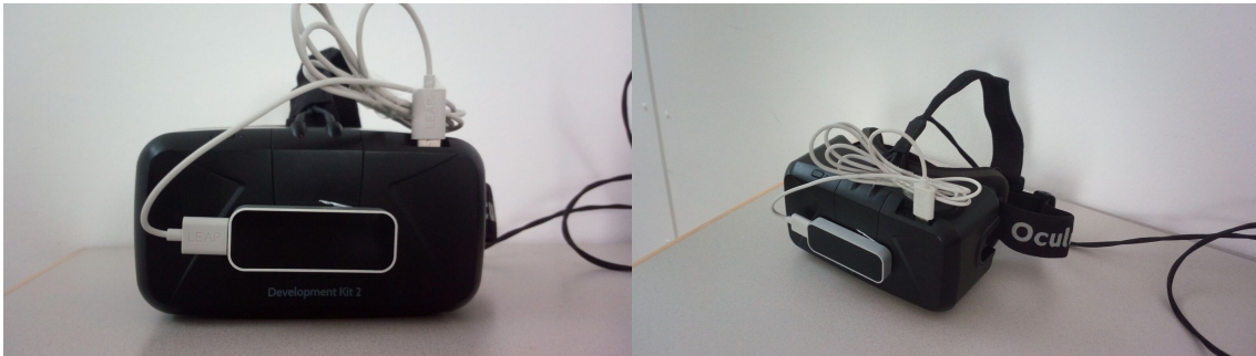
Figure 3.2: Hardware Setup: Leap Motion mounted on Oculus Rift DK2
