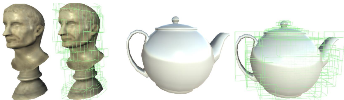
Figure 3.25: Physical object representation: low LoD
