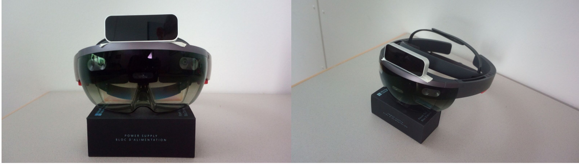
Figure 3.4: Hardware Setup: Leap Motion mounted on HoloLens
