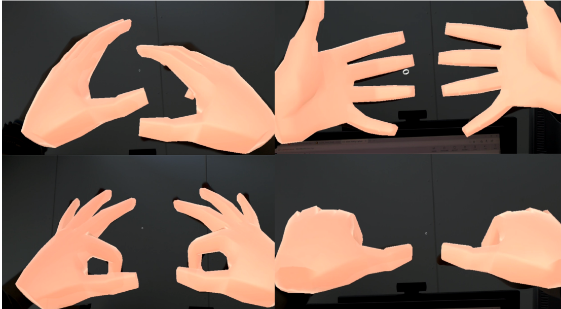
Figure 3.5: Alignment with virtual hands and real hands. The skin colored mesh aligns very close with the real hands which are consequentially barely visible. Different hand poses are presented with both hands simultaneously to show the fitting alignment of real- and rendered hands.
