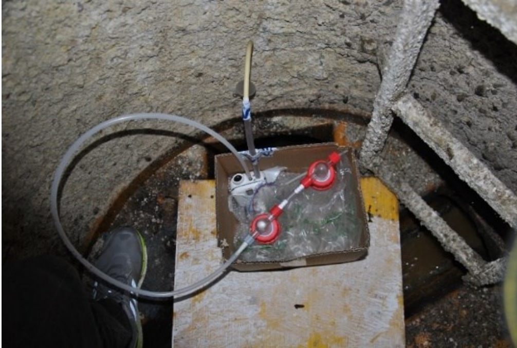
Figure 2: The device build for \text{H}_2\text{S} precipitation, including two interconnected Woulff bottles filled with a 0.1 \text{ M} silver nitrate or 5\% zinc acetate solution through which \text{H}_2\text{S} bearing sewer atmosphere was bubbled using a hydraulic aquarium pump.
