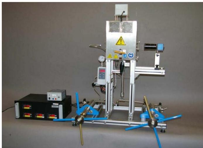
Figure 2. The High Pressure View Chamber Type HPVC 300-HT
