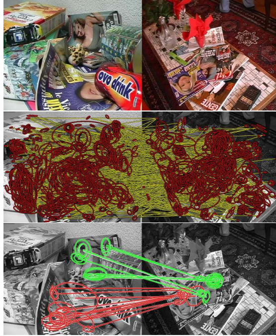
Figure 4.8: Cho et al. (2009) employ agglomerative clustering for the recognition of deformable objects. In their approach, the geometric deformation of objects is factored into the dissimilarity measure.
