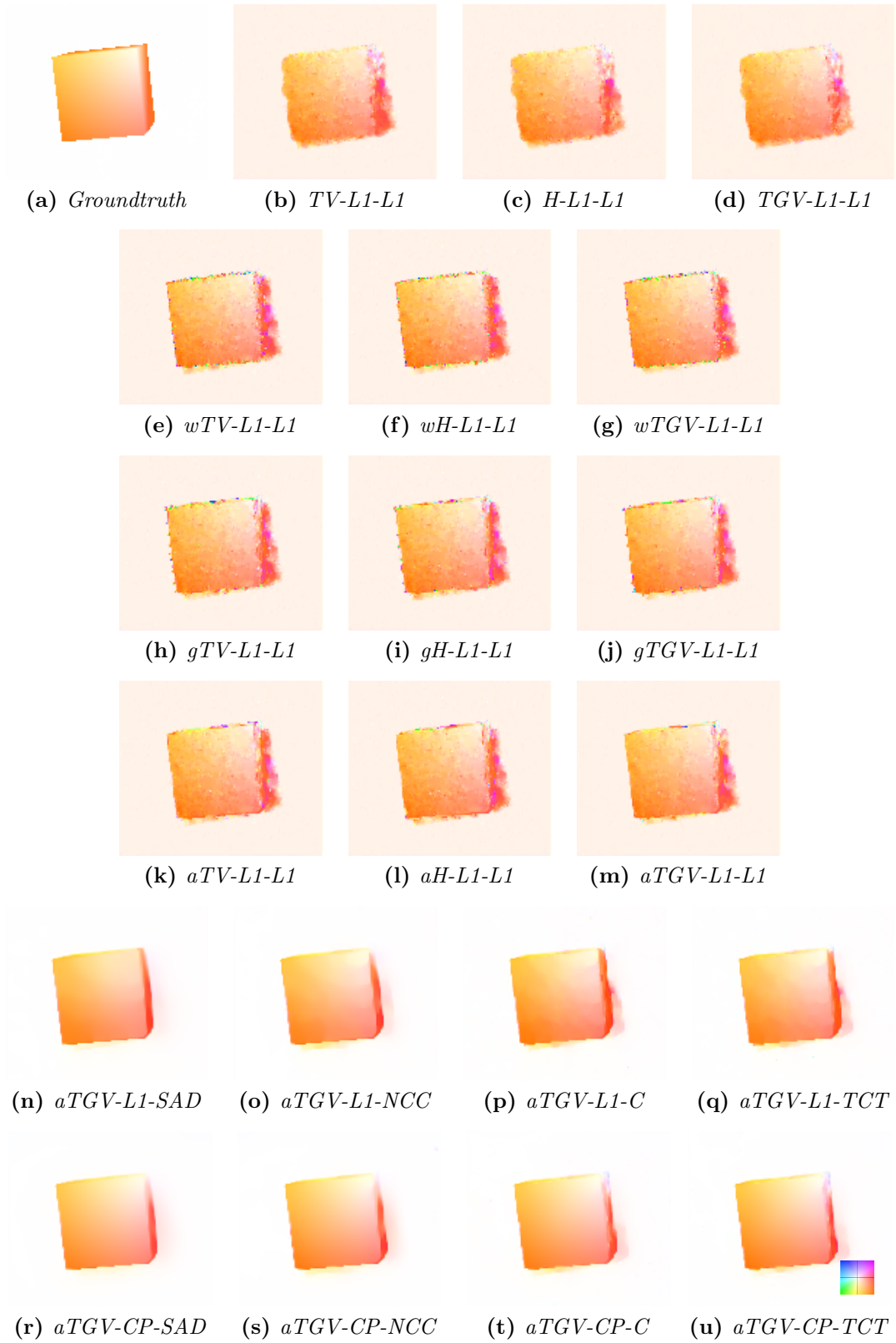
Figure 5.16: Flow estimation on a synthetic dataset for a rotation of 5 degrees about X , Y and Z and a translation of t = [10\%, 10\%, -10\%]^T of the object size. The color key is shown on the bottom right.
