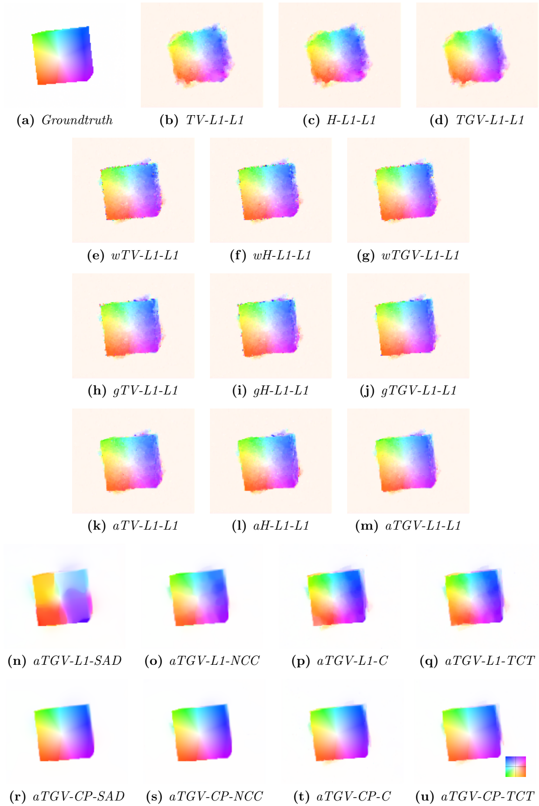
Figure 5.15: Flow estimation on a synthetic dataset for a rotation about the Z axis. The color key is shown on the bottom right.
