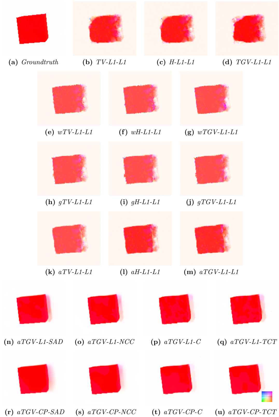
Figure 5.13: Flow estimation on a synthetic dataset for pure X translation. The color key is shown on the bottom right.
