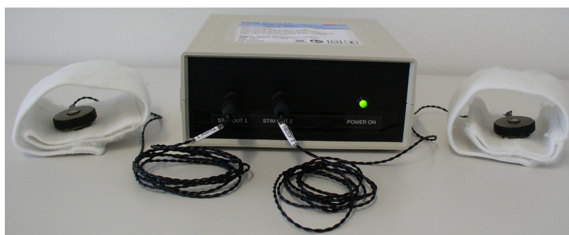
Figure 2.1.: Tactile stimulation device. The tactile stimulation device is shown with two C-2 factors connected. The factors can be attached to the left and right wrist using elastic wrist bands.
