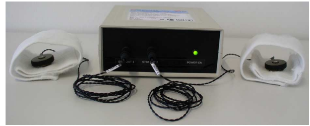
Fig. 4. Tactile stimulation device with two C-2 factors connected. The factors can be attached to the left and right wrist using elastic wrist bands.
