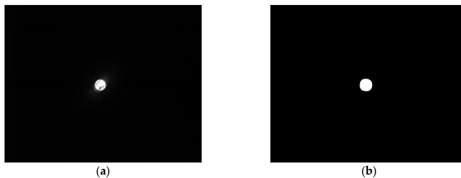
Figure 6. (a) Complete frame without image processing; (b) Complete frame with image processing to binary mode.
