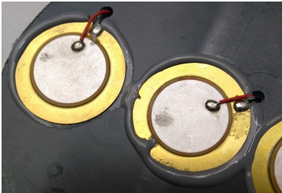
Figure 7: Epoxy resin glues piezo-elements
