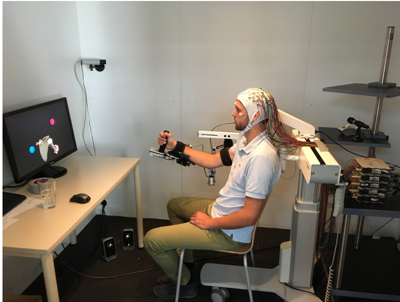
Figure 15: Experimental setup. A subject sitting in front of a screen which presented feedback. EEG electrodes mounted and connected to 5 USBamps.
