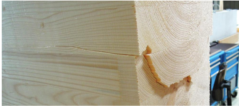
Figure B.2: Shear failure at the left end of specimen A04
