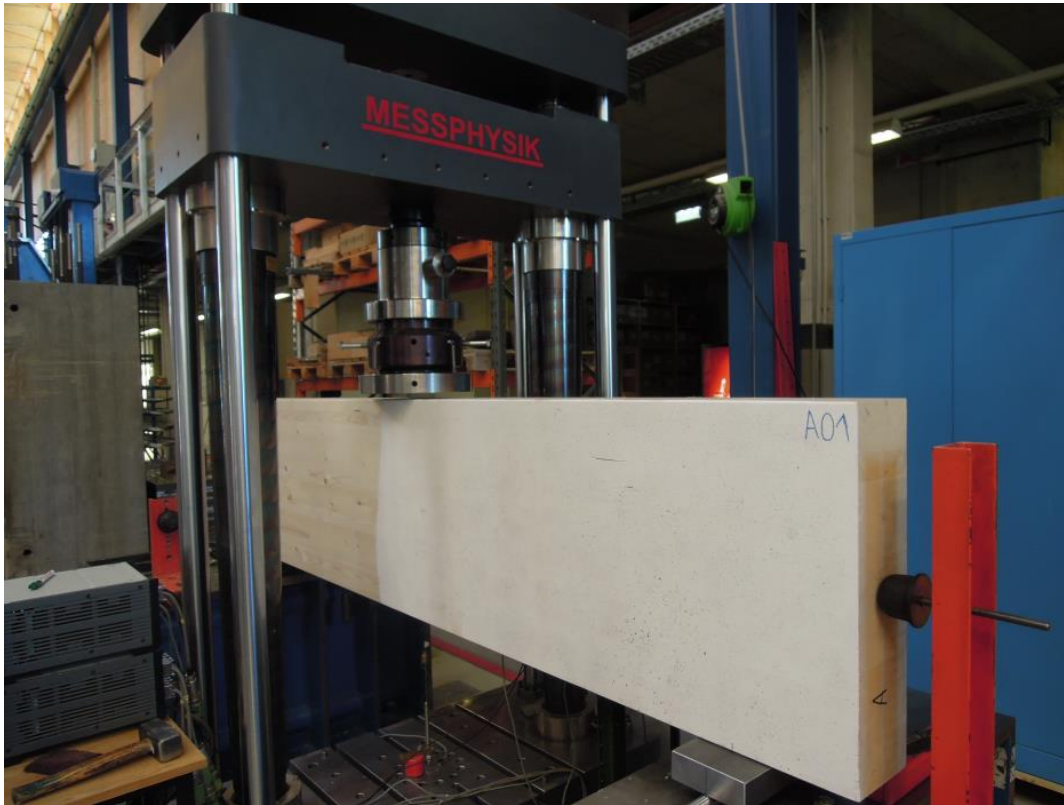
Figure 4.2: Test specimen A01 in the testing machine
