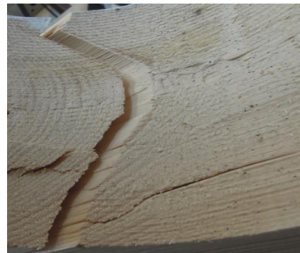
Figure B.14: Spreading of the crack through the opening vicinity on the upper left side (left) and lower right side (right) of specimen D01
