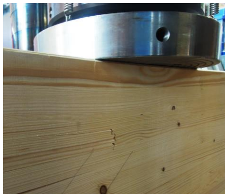
Figure B.30: Tension force influence on the beam back side of test specimen G02
