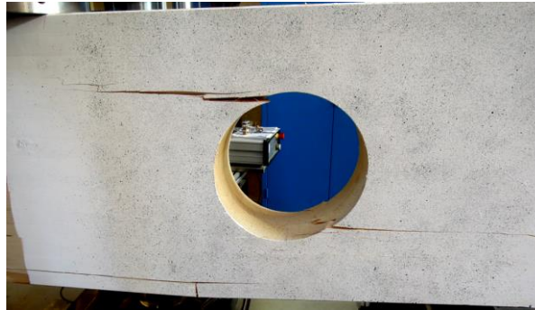
Figure B.17: Tensile stress perpendicular to the grain cracks on the upper left and lower right opening edge and bending crack of specimen D01
