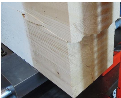
Figure B.15: Serrated shear failure on the right beam edge (left); the initial cracks on the lower right and upper left edge of the opening with additional crack and bending failure in the net cross section (right) of specimen D01
