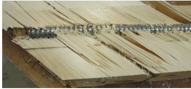
Figure B.34: Threaded rod hole with the threaded rod in the hole of test specimen G03
