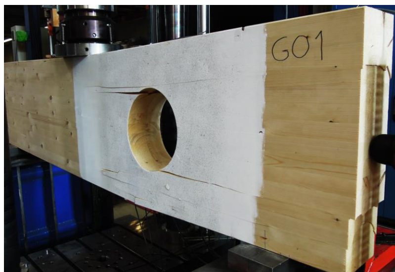
Figure B.26: Shear failures of test specimen G01
