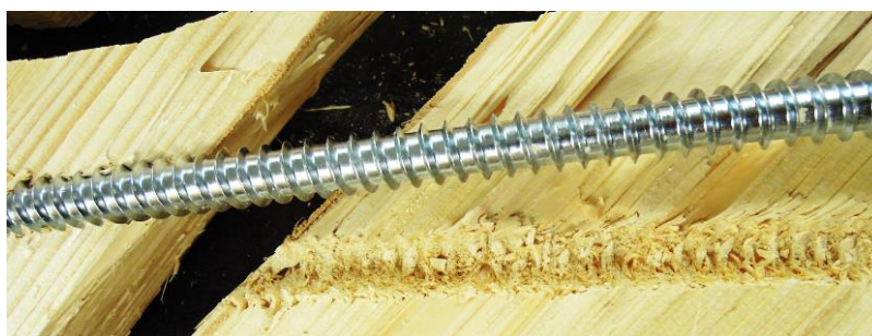
Figure B.21: Pull through effect by the threaded rod hole of test specimen D03
