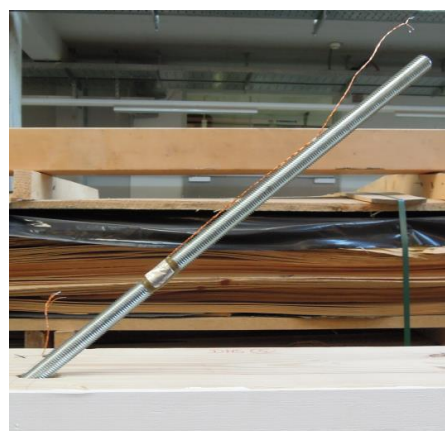
Figure 3.4: Series H; the strain gauge glued on a threaded rod
