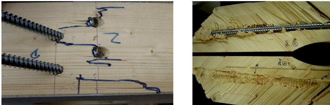
Figure B.16: Bending failure on the bottom side of the beam (left); threaded rod in the hole and pull through effect on the timber inside of the hole (right) of test specimen D01
