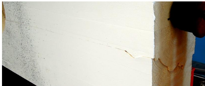
Figure B.4: Shear failure on the right edge of the beam of specimen B05
