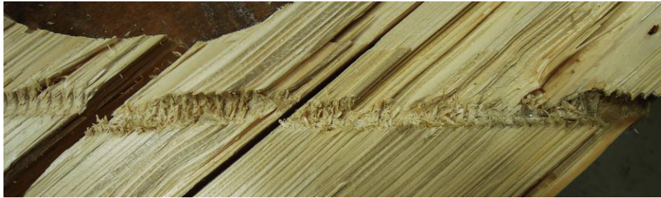
Figure B.32: Pull through effect of the threaded rods of test specimen G02
