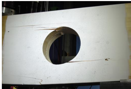
Figure B.29: Multiple cracking of the beam opening and bending failure in net cross section of the beam of test specimen G02
