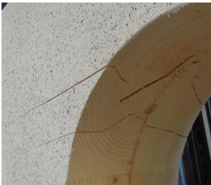
Figure B.7: Crack due to tensile stress perpendicular to the grain on the upper left opening edge (left) and on the lower right opening edge (right) of specimen C05
