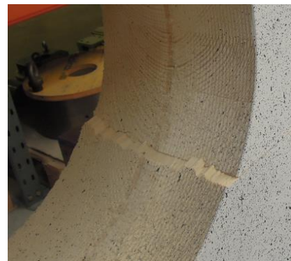
Figure B.7: Crack due to tensile stress perpendicular to the grain on the upper left opening edge (left) and on the lower right opening edge (right) of specimen C05
