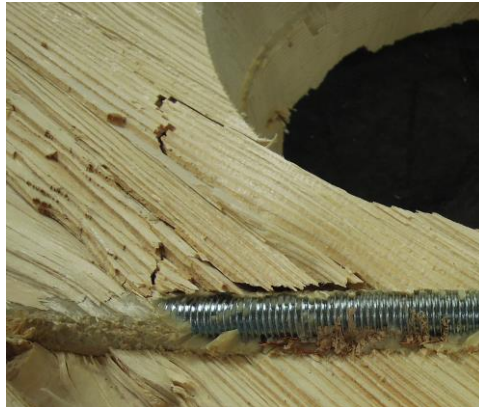
Figure B.41: Glued-in threaded rod inside of the damaged timber of test specimen H02
