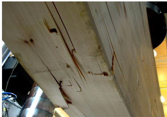
Figure B.10: Bending failure on the bottom side of the beam under the load application area of specimen C07
