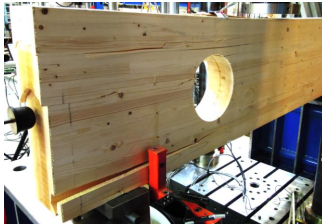
Figure B.37: Test specimen H01 back view with outbreak of timber part
