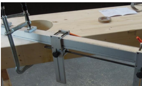
Figure 3.6: Drilling support rig from side (left) and from above (right)
