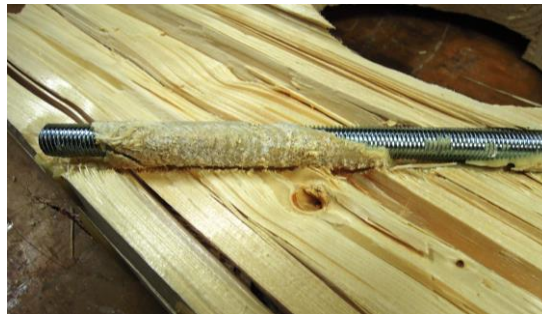
Figure B.39: Threaded rod inside of the hole with the glue on it of test specimen H01
