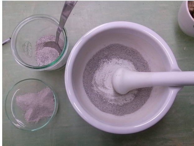
Abbildung 4.5: Concrete being ground up finely
