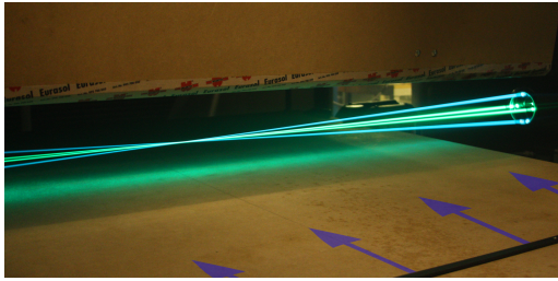
FIGURE 4. THE LDA SETUP TOGETHER WITH THE BLP, AP AND TRIPWIRE (FLOW FROM BOTTOM RIGHT CORNER)
