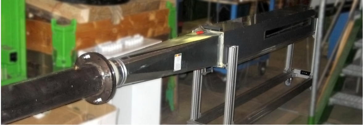
Figure 4.2: Photograph of the wind tunnel A2 showing the elongated diffuser, test section and optical access (flow from left to right) [110]
