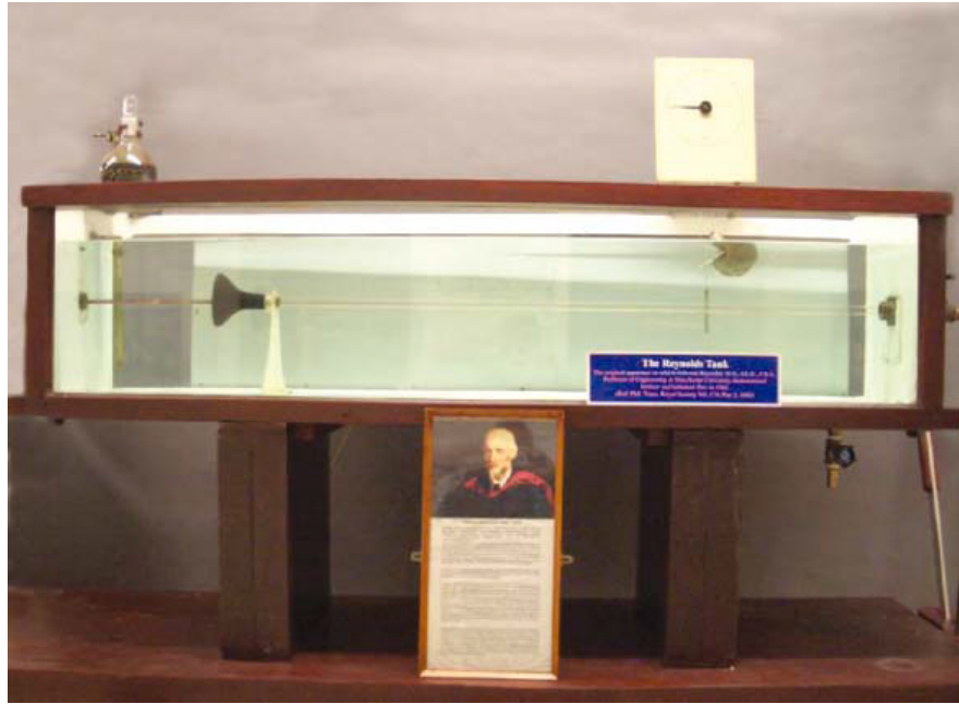
Figure 2.1: The original tank from the experiment of Reynolds at the University of Manchester [20]
