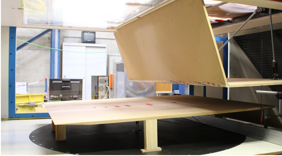
Figure 4.7: Photograph of the relaminarization test section in wind tunnel B , flow from left to right
