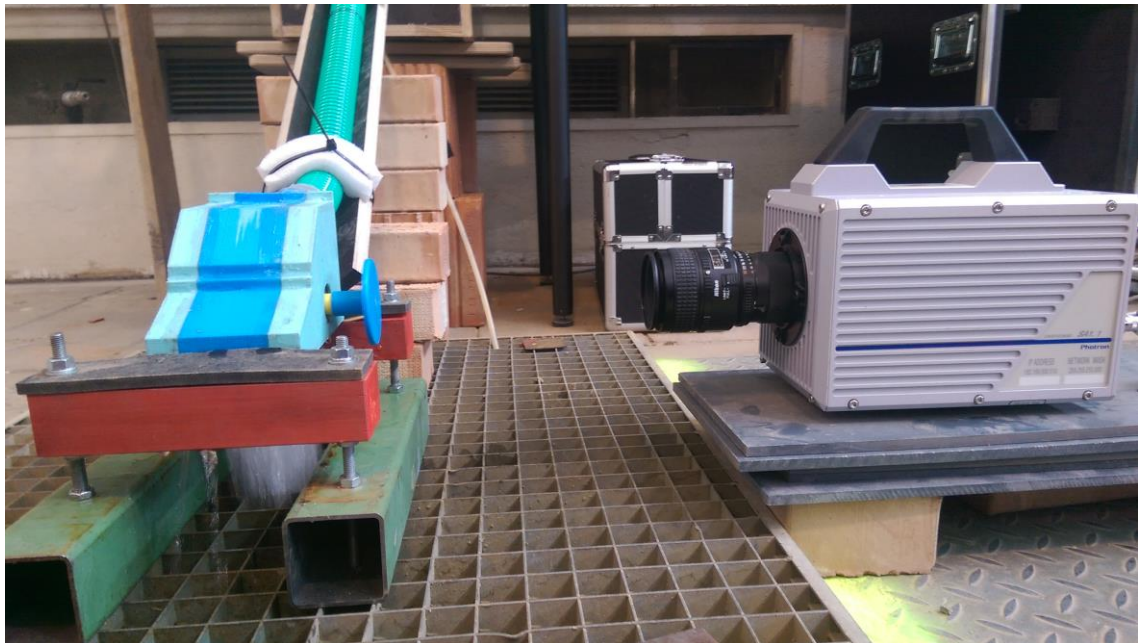
Figure 3-31: High-speed camera measuring the RPM of the turbine shaft.
