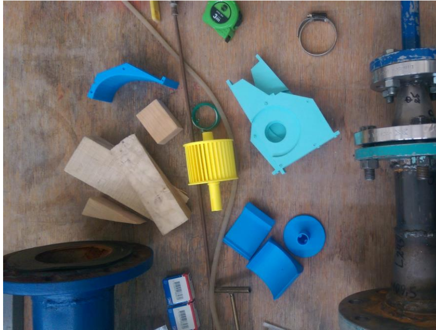
Figure 3-23: Turbine before the assembly; left and right sides of the housing in green, runner yellow and guide vanes in blue
