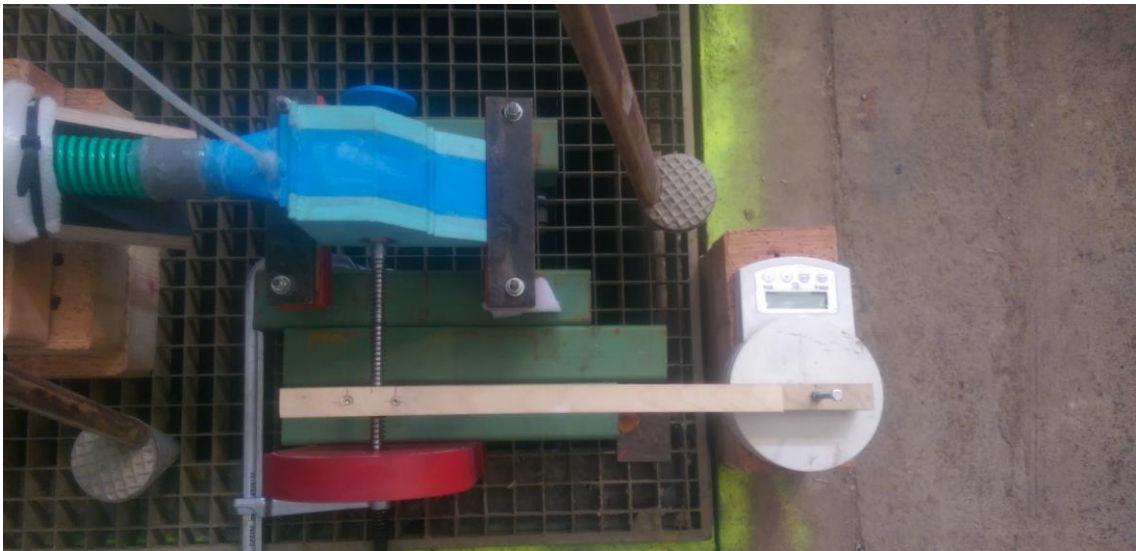
Figure 3-30: Prony brake mounted on the rotating shaft of the turbine runner
