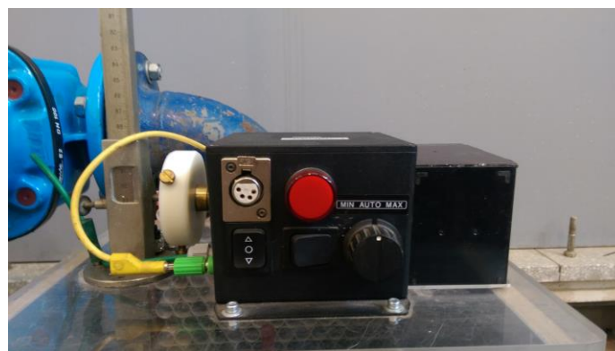
Figure 3-29: Measuring rod connected to the automatic handle for measuring the head
