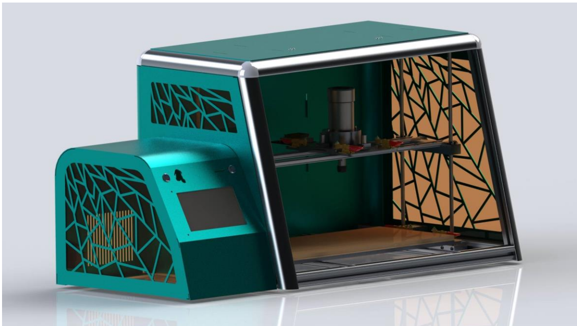
Figure 3-17: SheePEM CNC and 3D printing machine, capable of Printing 3D models as engraving and milling (Source; [6c])
