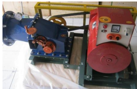
Figure 1-25: Belt drive system connecting the turbine left (blue) with the generator right (red) (Source; http://www.pme-bandung.com , 2012)
