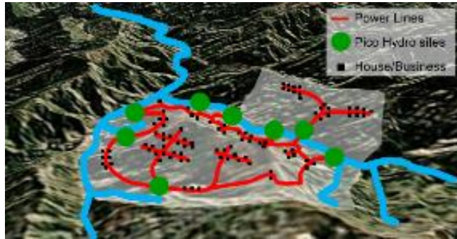
Figure 4-3: Pico-hydropower off-grid network concept, where each unit is exactly the same and the network expands as more units are purchased.
