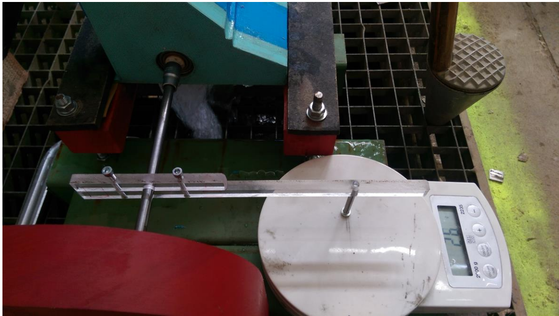
Figure 3-33: Measuring process of the turbine efficiency
