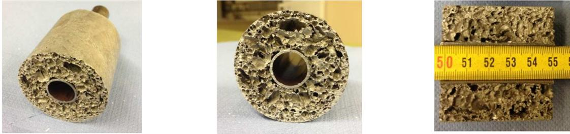
Figure 2-6: Internal structure of the aluminium foam
