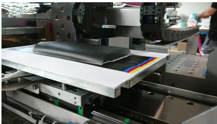
Figure 82. One sided wetting curl of pigmented paper right after printing
