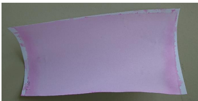
Figure 39. Wetted papersheet with dye ink as indicator.
