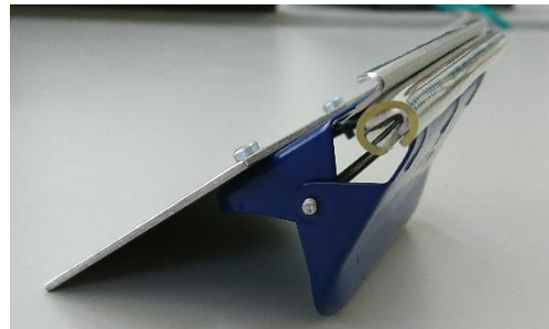
Figure 41. Picture of the lower clamp which has exactly 160 g
