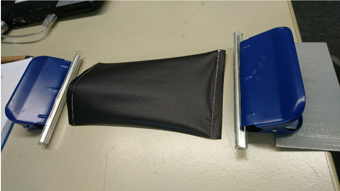
Figure 42. Result of the hot air drying experiment with 4x70 % ink and primer application
