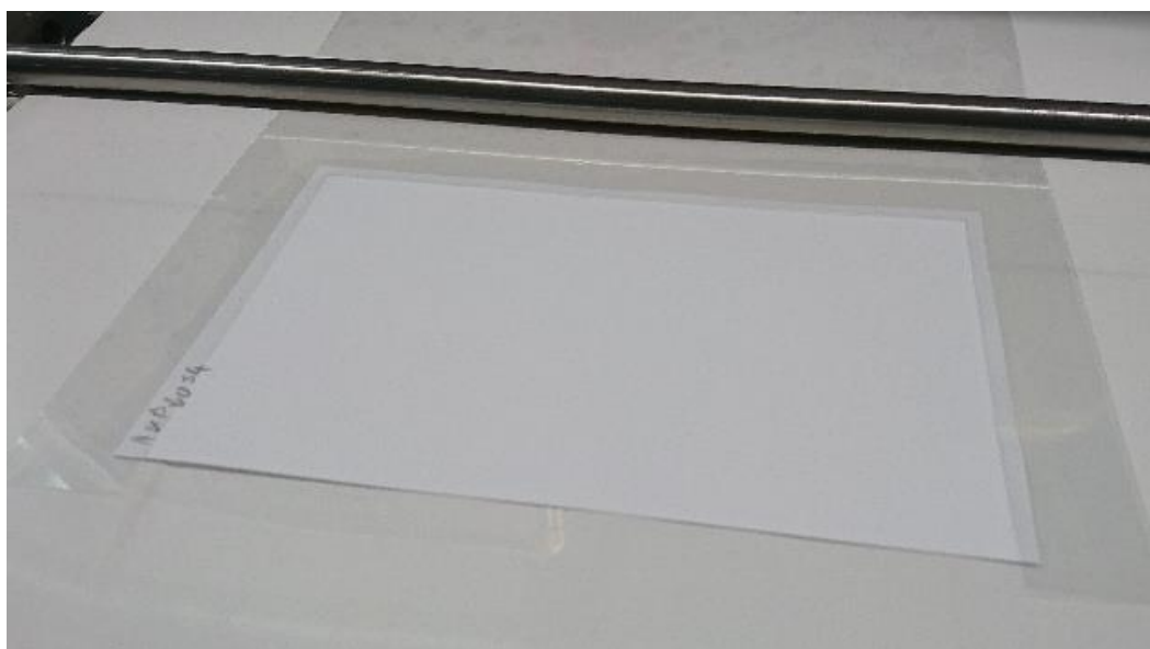
Figure 37. Paper sample for the rod coater. The sample is supported by a plastic film at the backside to allow easier transfer of the per-wetted sample to the IPTS. A second plastic sheet which is cut at the edges defined the area for the water application. Addition of a small amount dye ink helped in the pretrials to check the homogeneity of the water application.
