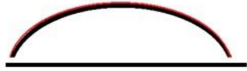
Figure 47. Sketch of a negative curl sample after printing. The red colour indicates the printed side.
