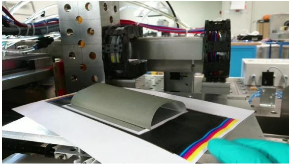
Figure 80. One sided wetting curl of AKD sized paper right after printing.
