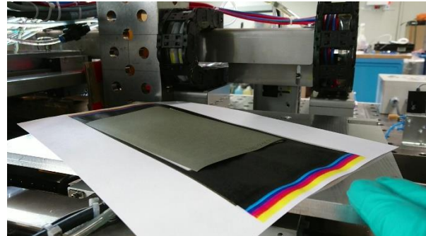
Figure 81. Collapsed AKD sample 21 seconds of free air drying.
