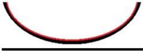
Figure 46. Sketch of a positive curl sample after printing. The red colour indicates the printed side.
