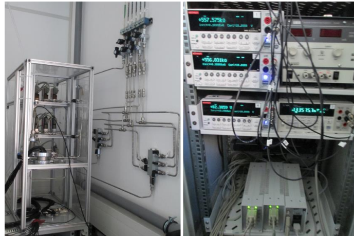
Figure 6.1: Automated gas measurement setup (on the left) with Source Measure Units (SMU) for electrical characterization and power supply for mass flow controllers (on the right).
