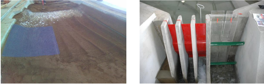
Figure 4.10: Physical model; left: installation of the river bed; right: detail view of the model outlet
