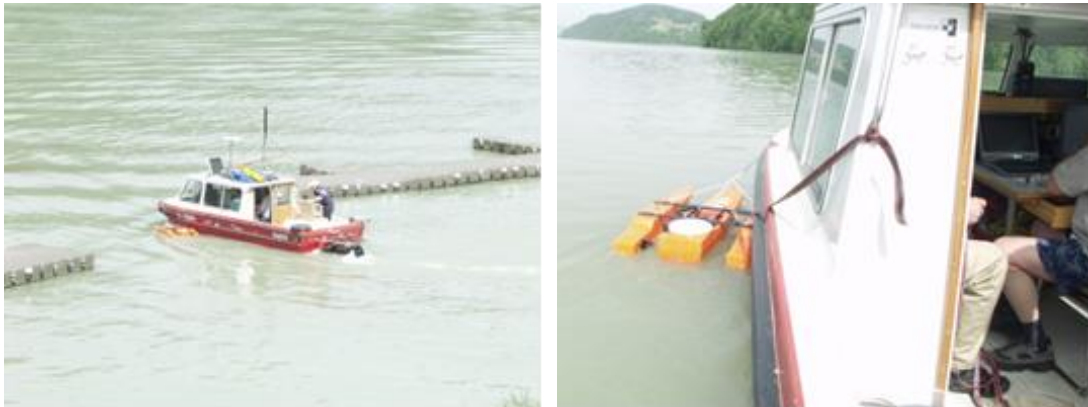
Figure 5.1: ADCP in action in the reservoir of the HPP Feistritz
