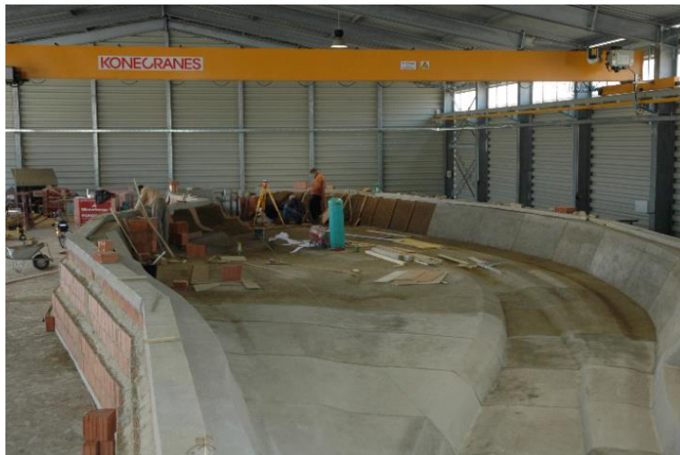
Figure 4.9: Photograph of the physical model under construction in the laboratory
