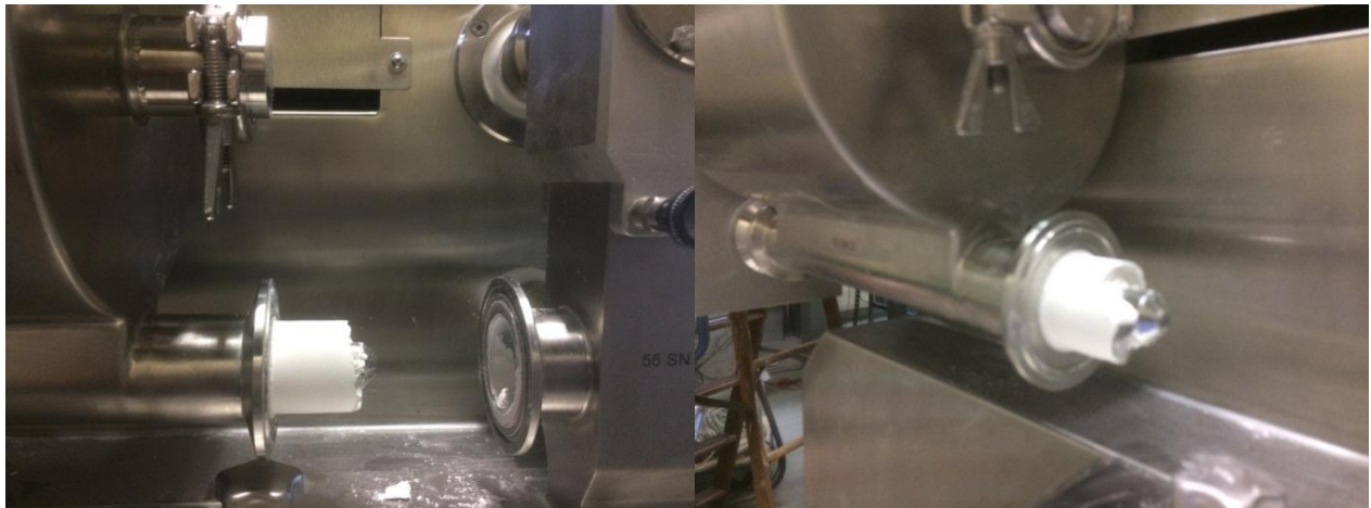
Figure 22: Avicel PH 105, stuck inside the feeding auger due to its cohesive powder properties, necessitated manual cleaning
