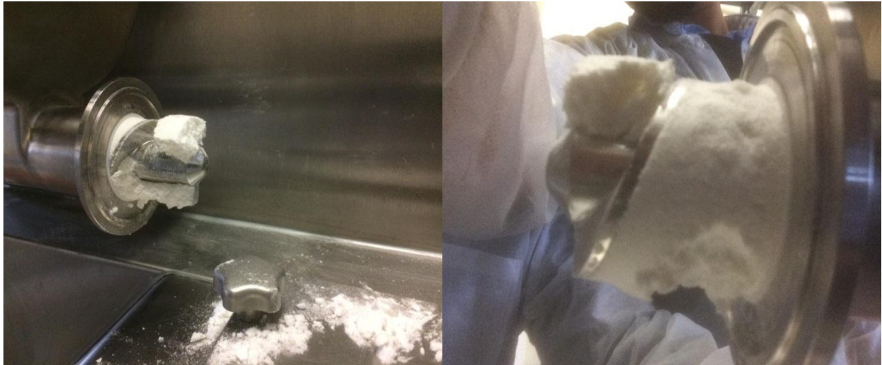
Figure 23: Solka Floc, stuck inside the feeding auger due to its cohesive powder properties, necessitated manual cleaning
