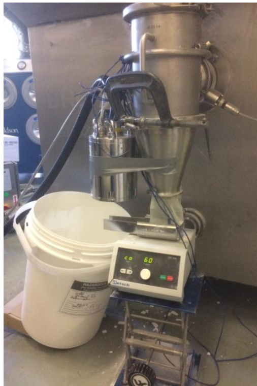
Figure 27: Setup for the roller compactor to collect test spectra of the created ribbons to improve the existing process monitoring model and to verify that built model.
