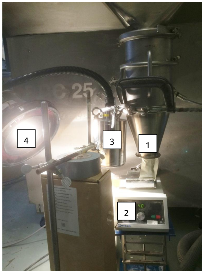
Figure 24: Setup for collecting NIR - spectra to build the calibration model. The main set up consisted of: 1) exit of the roller compactor, 2) vibrating feeder, 3) Matrix F from Bruker and 4) dust collector
