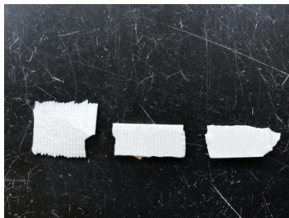
Figure 4: Ribbons from the top view, to see the irregularity and to understand why calipers are useless for determination of ribbons density
