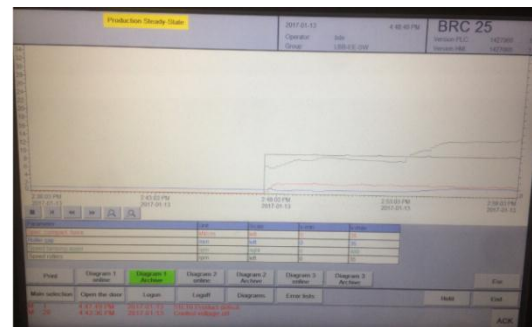
Figure 21: Process control of the BRC 25 to see the actual parameter values of the production. In addition, the time and the parameters of the whole production can be seen.
