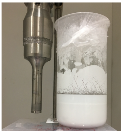
Figure 27: The sonicator probe and the boron nitride dispersion in a beaker glass. The sonicator tip should be well dipped into dispersion for an ideal distribution of the energy in the sample.
