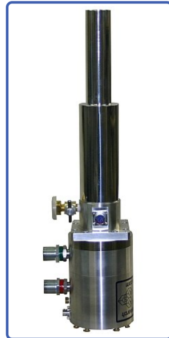
The above picture shows a cryocooler with a vacuum shroud, radiation shield, and sample holder installed.
