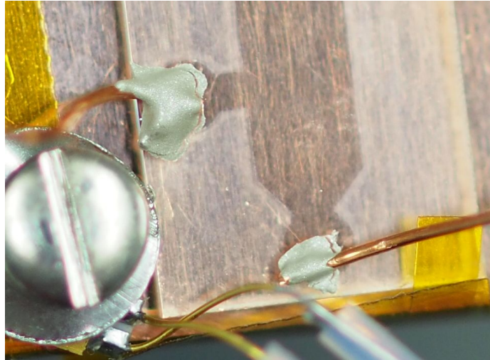
Figure 5.4.: Hairline fracture in the silver loaded epoxy adhesive at the contacts to the ITO Hall bar type structure.
