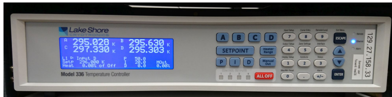
Figure 4.14.: LakeShore 336 temperature controller shown with disabled heating and cryostat at room temperature.
