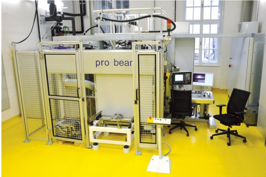
Figure 6: pro-beam electron beam welding machine K14
