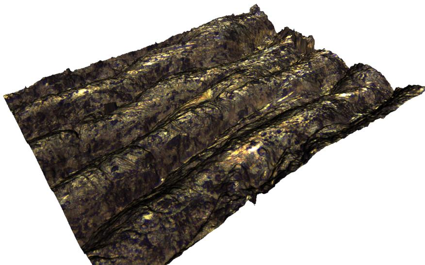
Figure 42: Alicona 3D surface picture of magnesium (line spacing = 0.25 mm, frequency = 10000 Hz)
