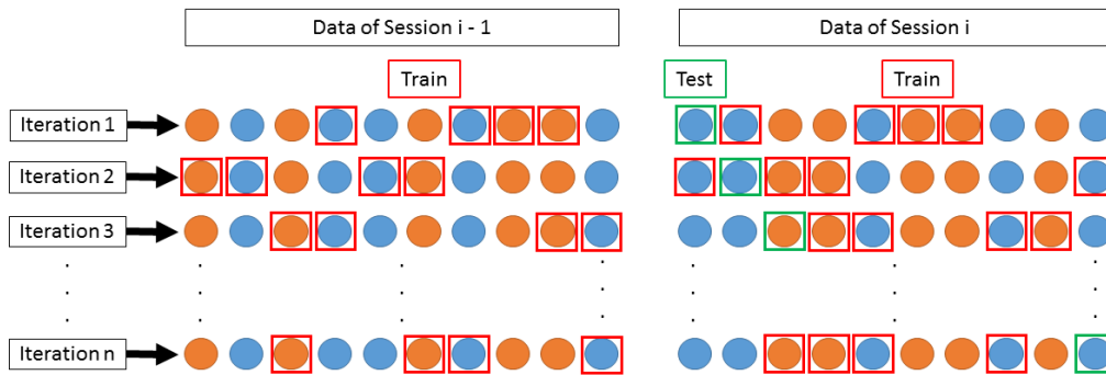
Figure 2.11.: Basic principle of the LOOCV applied in the case of data transfer. Test data is only taken from the current session. Training data is taken from the current and from the previous session to mimic the data transfer.
