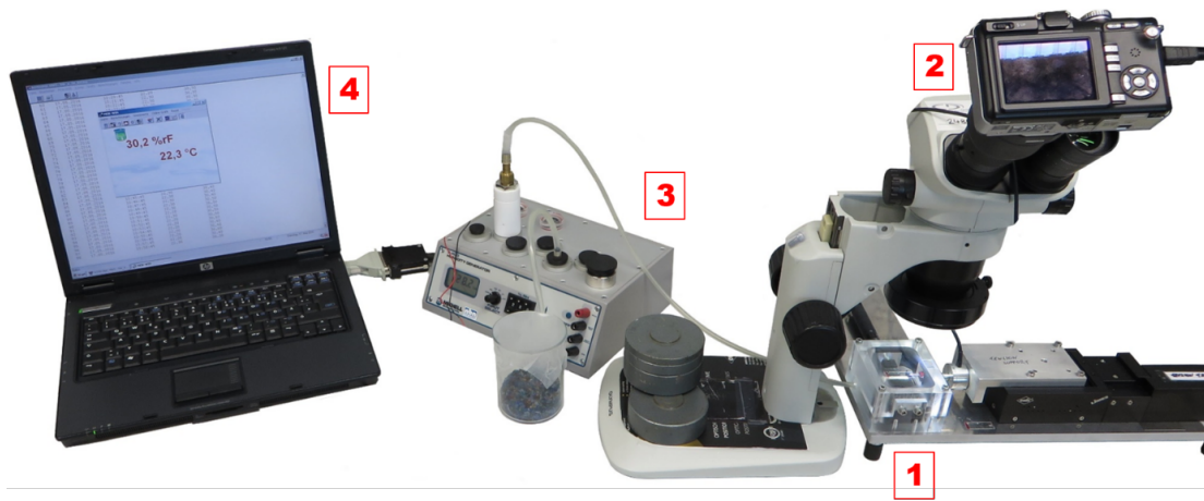
Figure 3.11 RH chamber testing setup: 1 - conditioning chamber, 2 - video camera, 3 - humidity generator, 4 - RH recording
