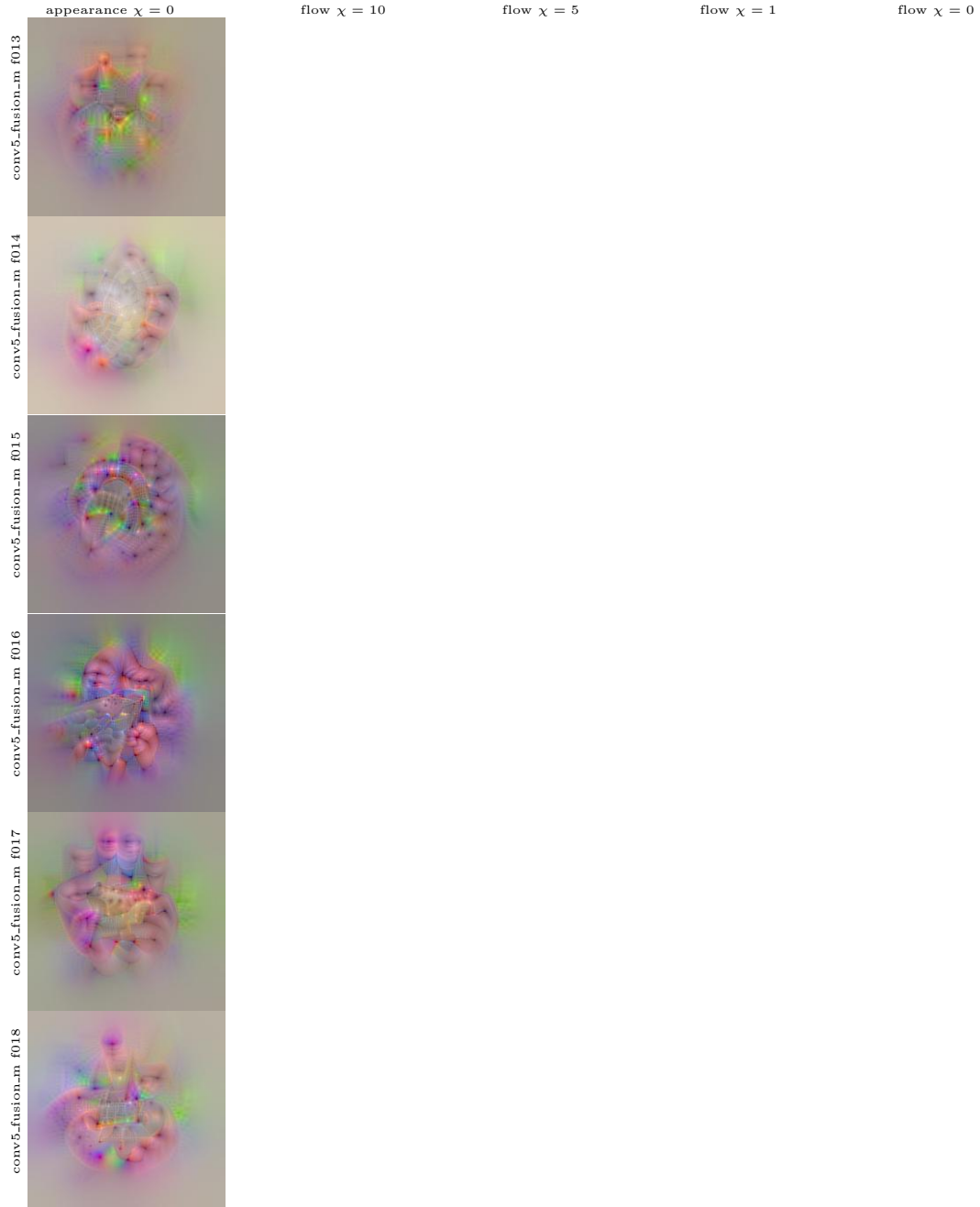
Figure B.15: Visualization of 6 filters of the conv5_fusion (motion stream) layer under different temporal TV regularization. We show the appearance input and the optical flow inputs for slowest \chi = 10 , slow \chi = 5 , fast \chi = 1 , and unconstrained \chi = 0 , temporal variation regularization.
