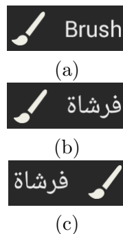
Figure 13.6: Screenshots for elements' positions in the tools dialog: (a) Original version (b) Incorrect position (c) Correct position .
