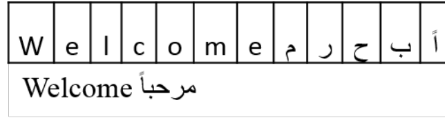
Figure 6.1: Arabic text (bidirectional) where the logical order in the first row and the visual order in the second row are not of the same sequence of characters.
