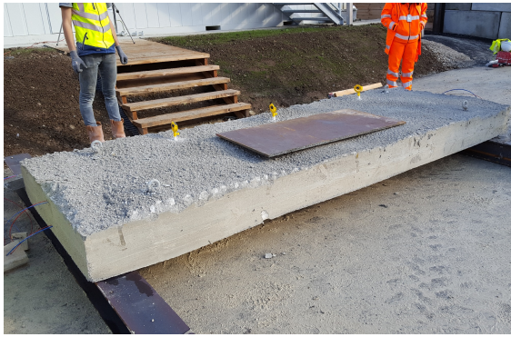
(a) Steel plate for load distribution.
