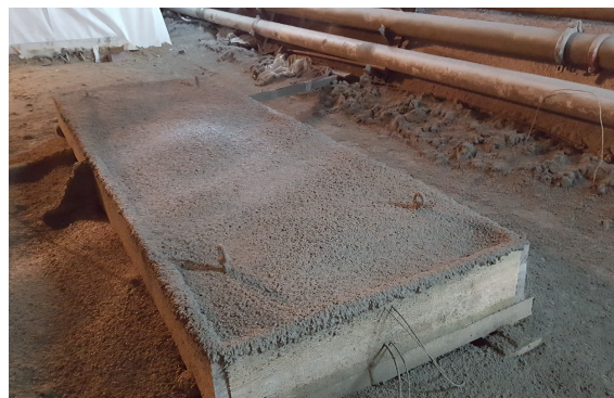
(f) Finished test slab with transport hooks.
