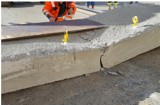
(c) Failure of the test slab.
