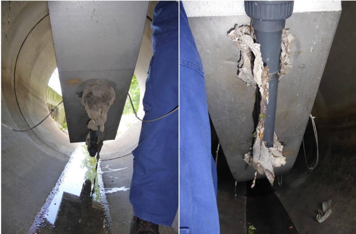
**Figure 2-25: Clogging of the cladding tube in which the spectrometer probe is installed after an overflow event (Photo: Hofer, 2016)**
