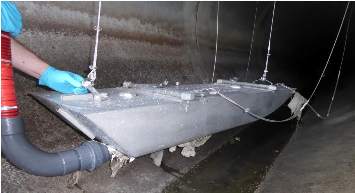
**Figure 2-24: Side view of the floating pontoon in Graz-WWTP-CSO where the spectrometer was installed after an overflow event (Photo: Hofer, 2016)**
