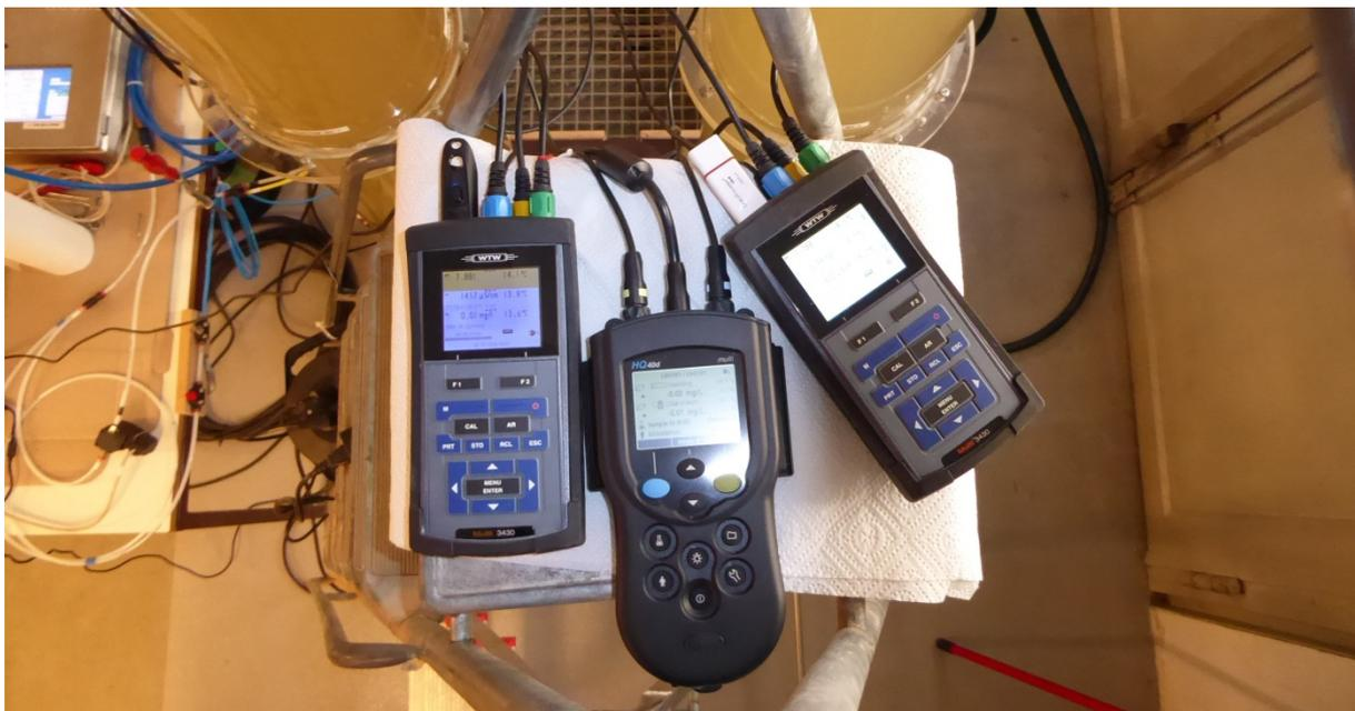
Figure 2-4: Used control units for secondary probes designed for laboratory use
