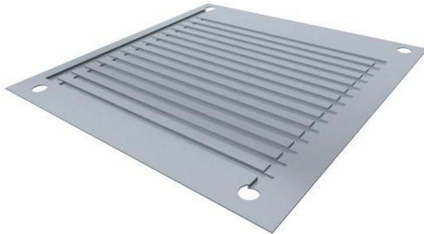
Figure 12: Concept of a bipolar plate made from thin metal sheet with flow fields on both sides. The inlet and the outlet is realized by circular holes. For both sided use additional sealing elements are required to give shape to the flow field channels next to the inlet and outlet.
