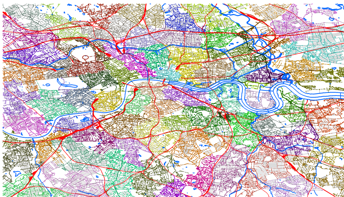
Figure 4.33: CRP partition of the London City Center ( 30 \times 17 km) road network (black) with waters (blue) and railways (red) shown on top of it.
