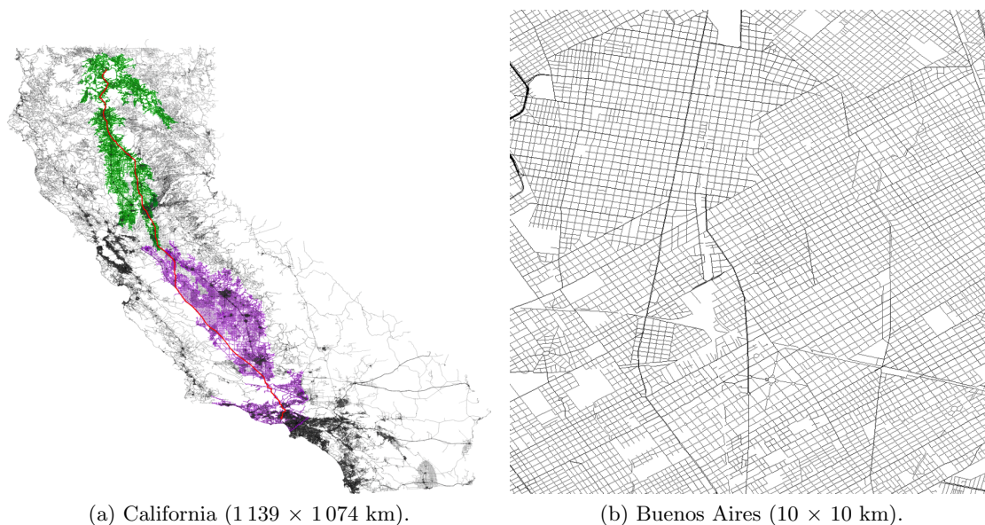
Figure 5.6: Road network of California with a bidirectional A* search and a section from the road network of Buenos Aires.
