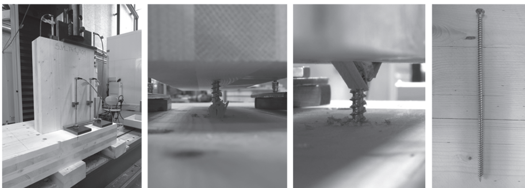
Figure 5.24: test configuration applied for a tension loaded fully threaded screw in a wall-to-floor joint (internal designation S_V1_T41)
