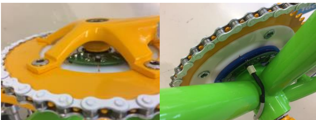
Figure 63: Chain wheel with antenna and tag PCB / reader mounted on frame
