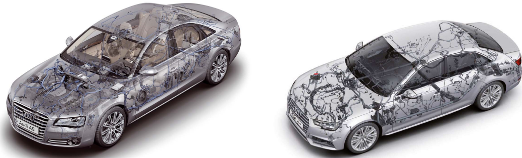
(a) Audi A8 Electric wires diagram. Picture extracted from [3]
