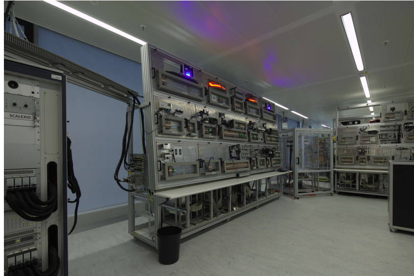
Figure 2.5.: Exemplar picture showing a classic HiL test bench, copyright AUDI AG
