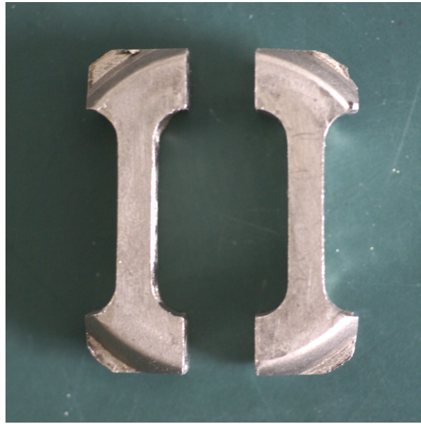
Figure 4.5: Two tensile test samples were cut from the disc specimen Ni10Ten. One of which was elastically deformed ('Ni10Ten') and one which was not ('Ni10NTen'). Difference dilatometry samples were cut from the two tensile test samples.
