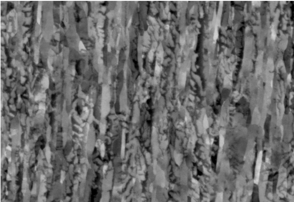
Figure 4.10: Scanning electron microscopy image of high-purity nickel deformed by HPT and subsequent cold rolling (specimen Ni16CR). The image shows the A-T plane of the specimen. The image width is 5.72 \mu\text{m} .
