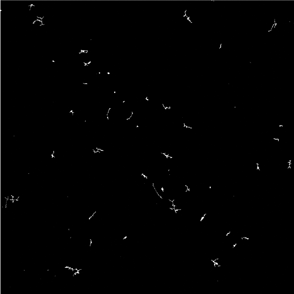
Figure 5.2: STEM-HAADF image of the covering rate of gold nanowires on an amorphous carbon grid. The nanowires are synthesized at T_{CH} = 5.4 \text{ K} with three different \alpha = \{0.75, 0.25, 0.1\} . A total mass of m = 0.8 \cdot 10^{-2} \frac{\mu\text{g}}{\text{cm}^2} is deposited on the TEM substrate, resulting in a coverage of roughly 0.8%.
