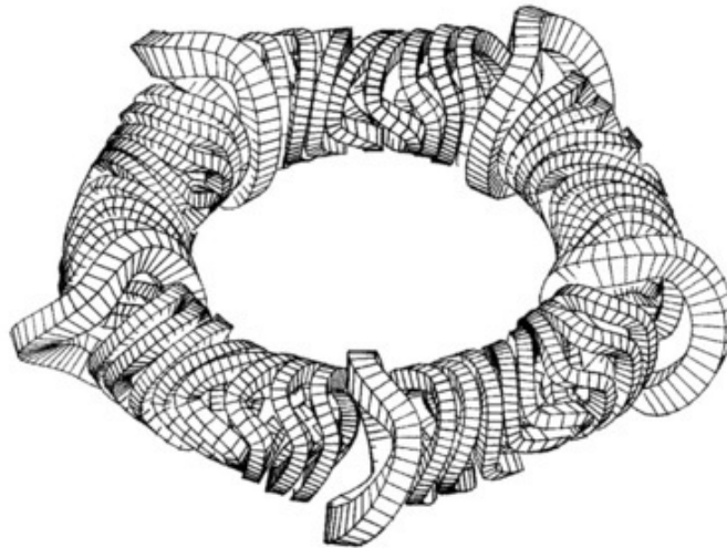
Figure 2.8: Coil system of the first optimized stellarator Wendelstein 7-AS. Figure taken from [60].
