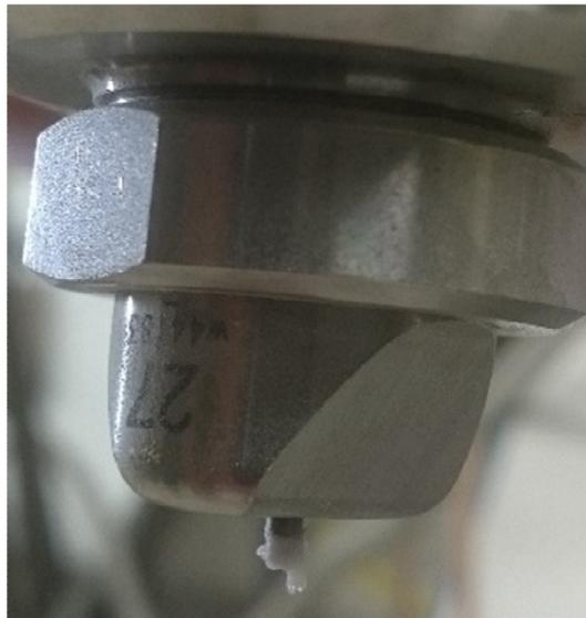
Figure 43: Blocked nozzle.
