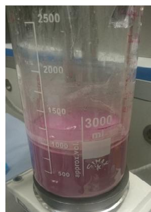
Figure 21: Iron-(III)-oxide spraying suspension (10w%)
