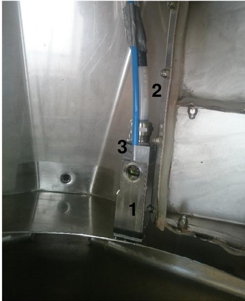
Figure 7: Final position of the OCT-Sensor (1) beneath the drum. The optical fibers are protected by surrounding hoses (2). To avoid dusting of the sensor window pressurized air is installed to protect the glass window (3).
