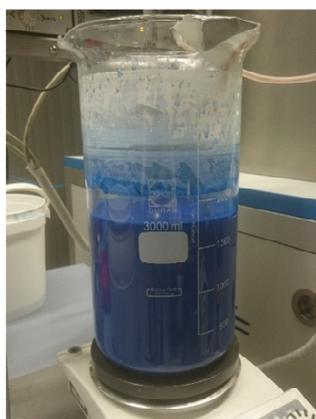
Figure 20: Indigo carmine spraying suspension (2w%)
