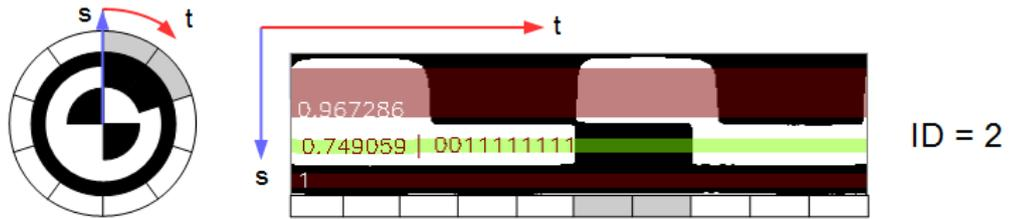
Figure 60: 3D Fiducial Propeller marker – the variation of  $s$  and  $t$  can be used to create a mapping for the  $x$  and  $y$  direction. The remapping of the marker results in a rectangular image that can be used to extract the marker identification (adapted from [56]).
