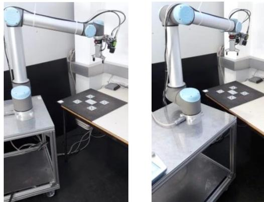
Figure 4: Significant change of the mobile platform pose at the workstation. Nevertheless, the robot should perform accurate pick and place operations
