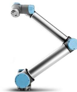
Figure 70: Visualization of the Universal Robot UR10 [65]
