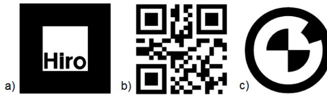
Figure 16: Marker types – a) 3D ARToolKit square marker [1]. b) 2D QR Code marker. c) 2D Fiducial Propeller marker (adapted from [56])
