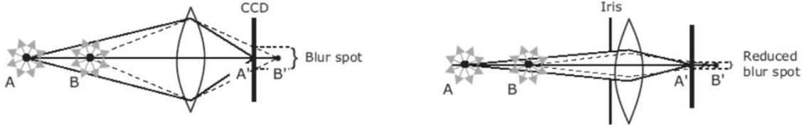
Figure 18: Influence of a changing amount of iris aperture on the blur spot of the image [57]
