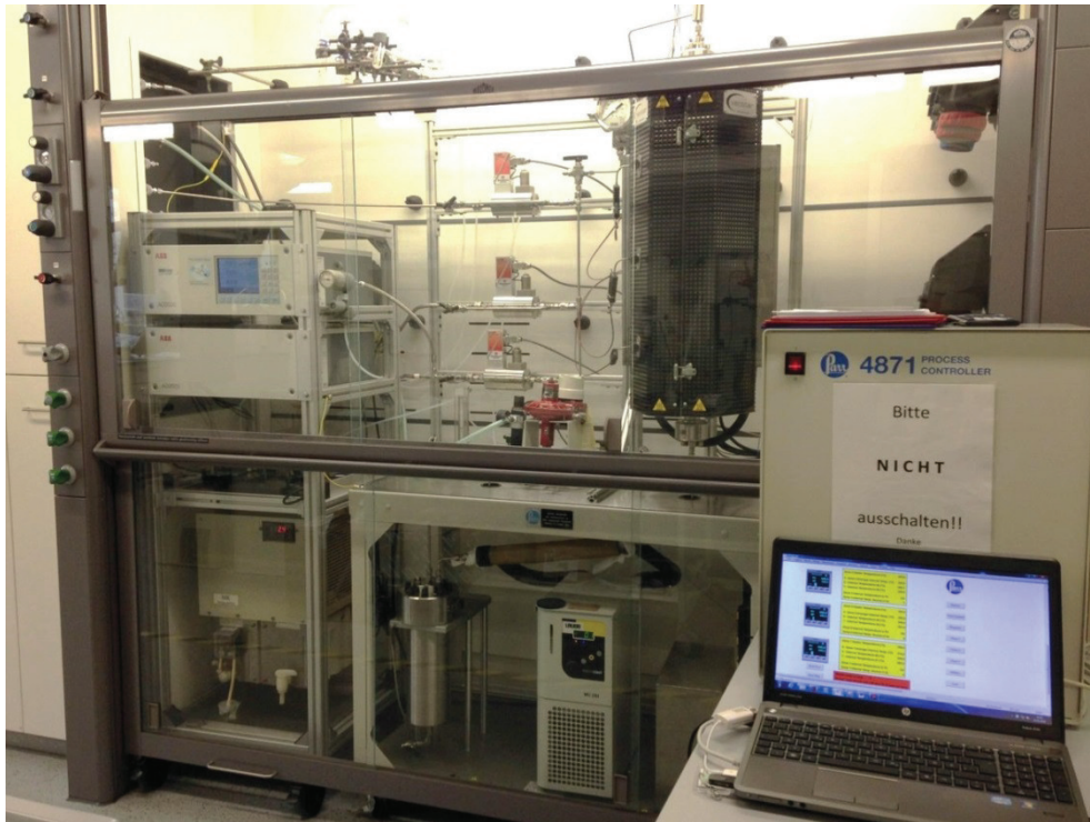
Figure 4-4: Picture of the tubular reactor setup [4] including (from left to right) the online gas analyzer, condensing vessels, double pipe heat exchanger with cryostat, reactor furnace, and process controller.
