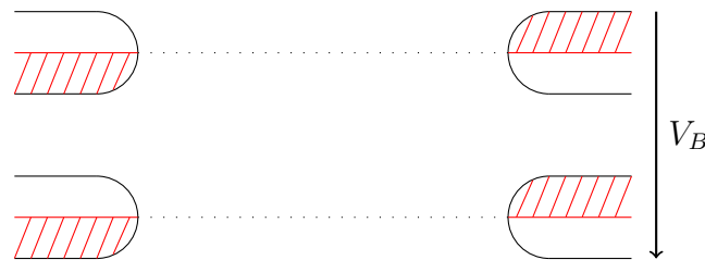
FIGURE 4.2: The position of the chemical potential in the energy space is denoted by the red line. The band is half-filled in that case, meaning the chemical potential is fixed relative to band.
