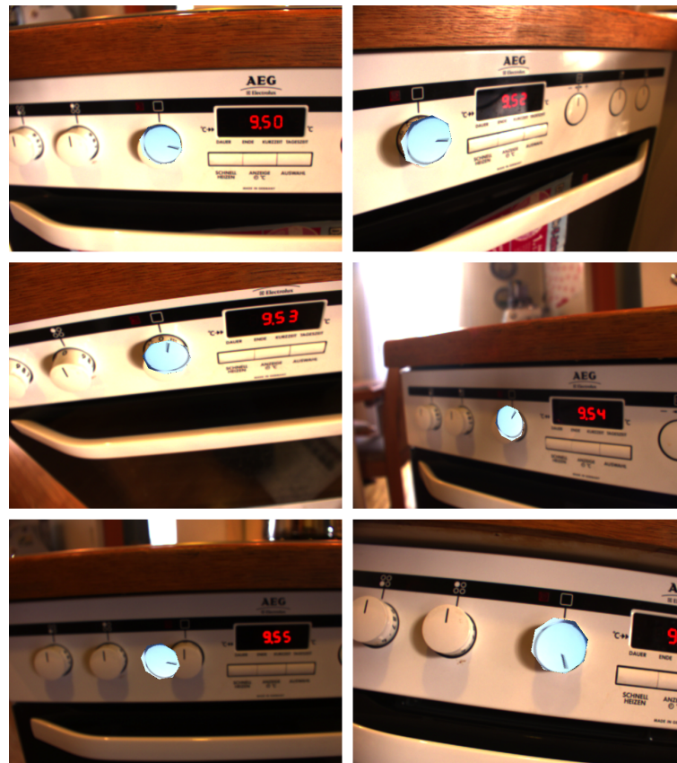
Figure 5.19: This series of pictures shows the poor results of bad lighting conditions. While the tracking had already problems due to the very bright and reflecting surface in the first three pictures, it totally failed when the lighting conditions were changed.
