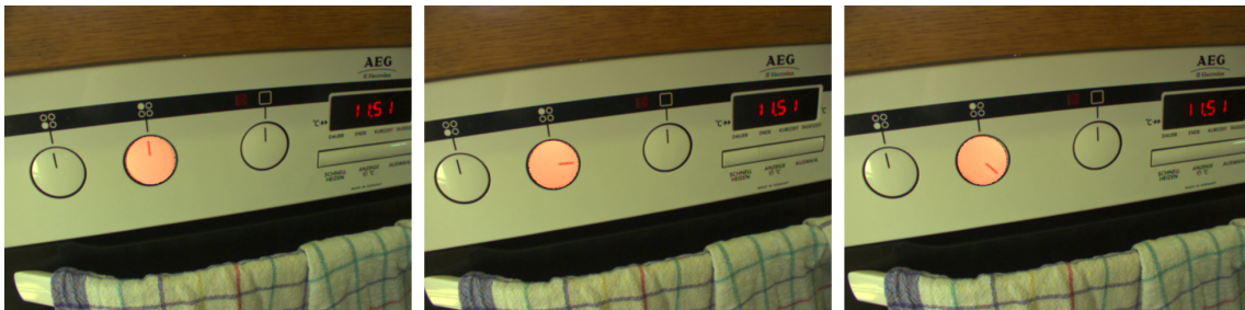
Figure 5.12: This figure depicts the progress of the applied, revolving control element on one of the temperature regulators.
