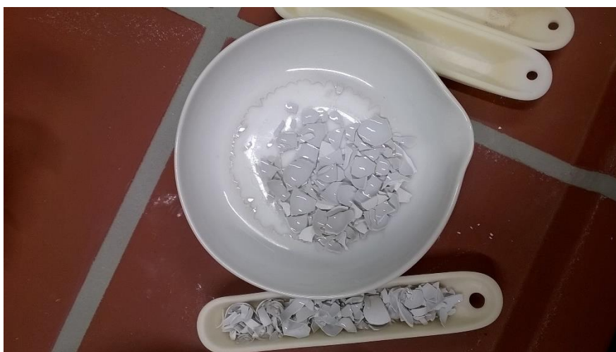
Figure 11 Multistep Sintering Sample after evaporation of 2-propanol prior to 900°C heating step
