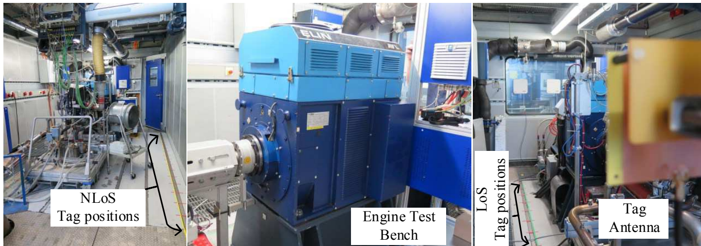
FIGURE 2.4: Engine test bed environment. Both of the LoS (green tape) and the NLoS (yellow tape) trails are shown in the figure, with red tapes depicting the position numbers.
