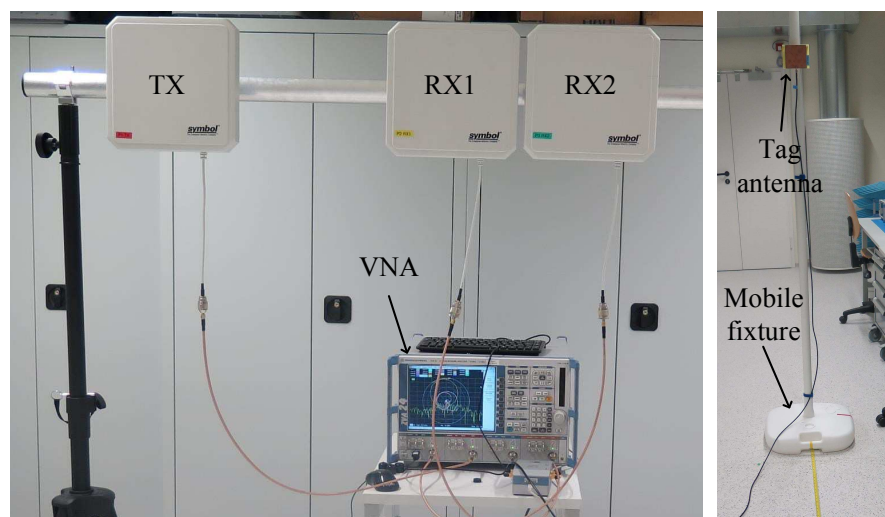
FIGURE 4.3: The antenna setup for the measurements. The measurement reference plane is at the input of the antennas. The origin is taken in the middle of RX1 and RX2 antennas. The gap between RX1 and RX2 is kept 27 cm. The distance between the TX and RX2 is 55 cm. The tag antenna was surmounted on a mobile fixture, so that it can be positioned freely in the IHF lab. The VNA generates continuous sinusoidal waves (without modulation) for the channel measurements. The frequency sweep range is from 600 MHz to 1.2 GHz.
