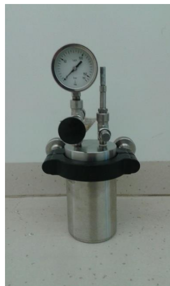
Fig. 16: Stainless steel autoclave for hydrothermal synthesis
