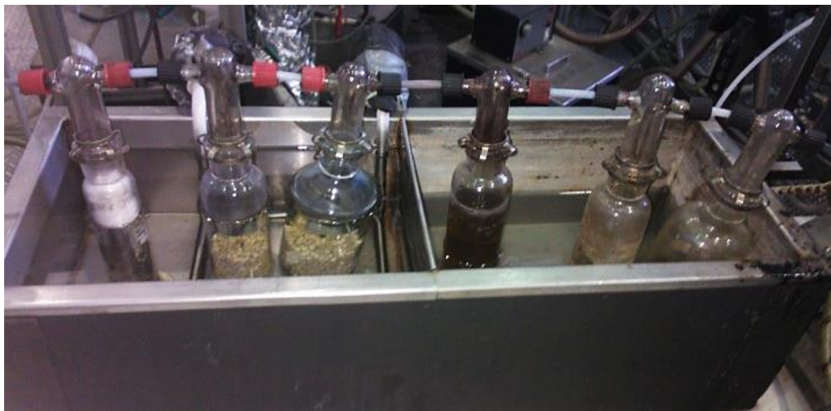
Figure 5-10: Impinger bottles for gas cleaning – 2 x water, 1 x RME, 2 x isopropanol, 2 x glass wool (only first one shown)
