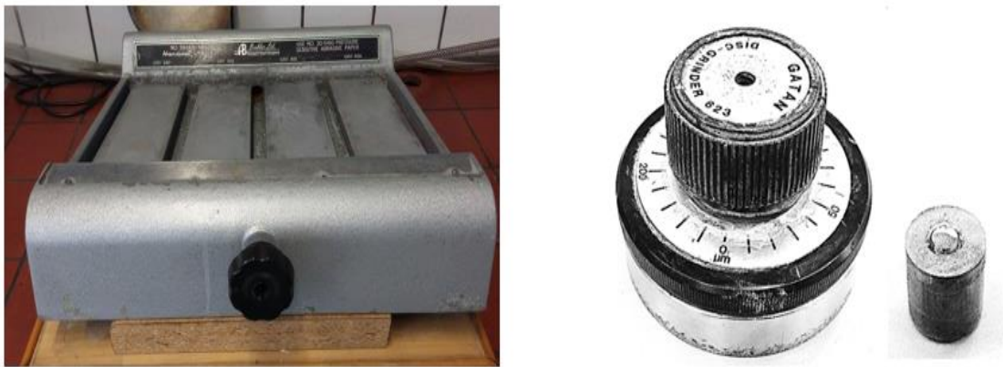
Figure 15: Buehler Handimet Grinder (left), Gatan Disc Grinder and support cylinder with sample (right).
