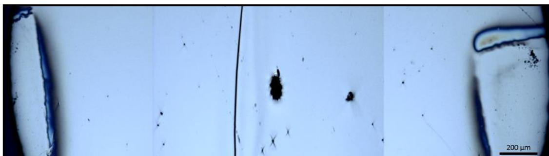
Figure 40: Overview of a light microscopy image of the Si_Ddw_1 sample. A tungsten wire is glued perpendicular to the clamps at the PIPS™. Fewer artefacts are visible on the sample surface and one big hole appeared.
