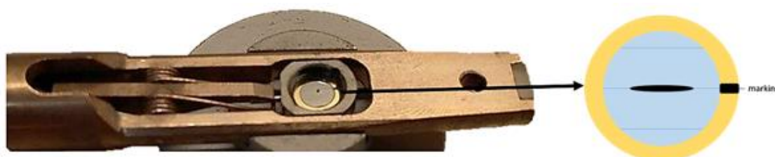
Figure 50: The position of the marking on a cross-section sample in the TEM sample holder.
