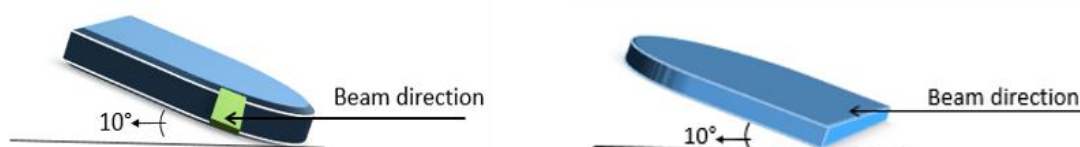
Figure 65: Usual milling conditions for FIB lamellae (left), test on Si sample with +10^\circ tilt (right) to simulate the conditions for AFM measurements.
