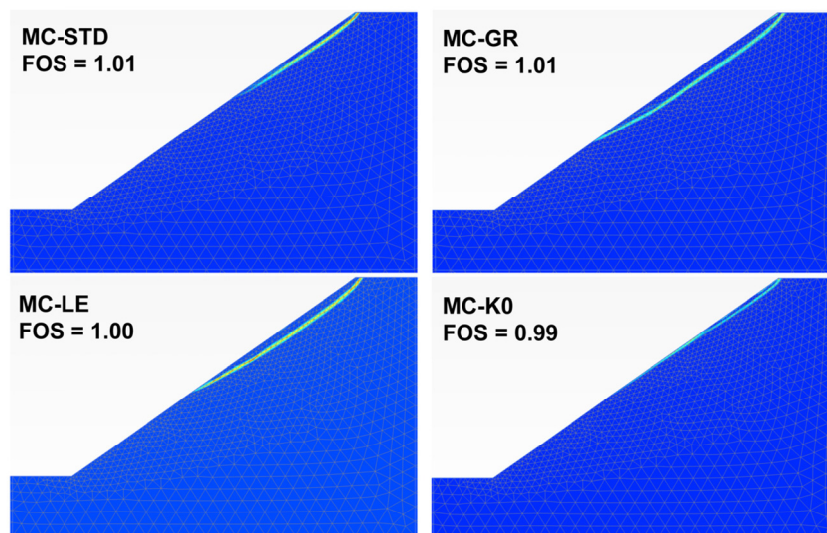
Fig. 32 Incremental deviatoric strain on a slope with \beta = 35^\circ and c = 0 kN/m 2 based on the user-defined material model
