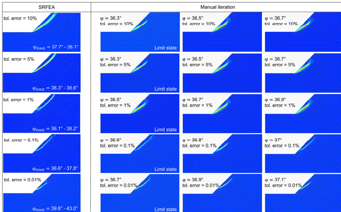
Fig. 42 Incremental deviatoric strain at limit state - manual iteration
