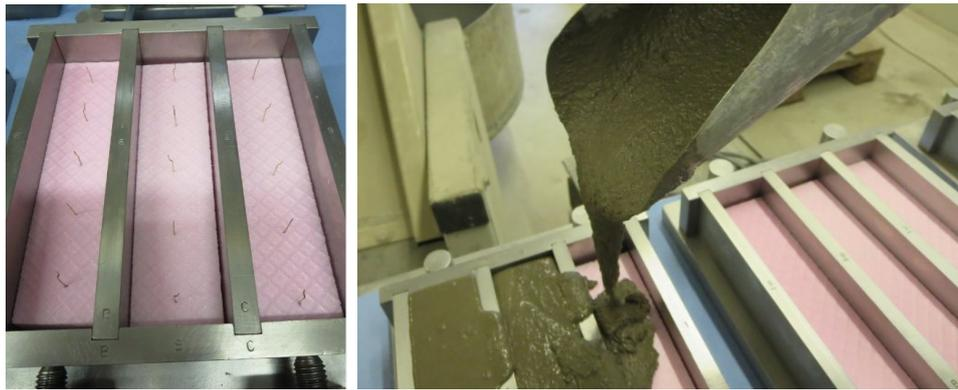
FIGURE 6.4.: Specimens preparation for pullout test.
