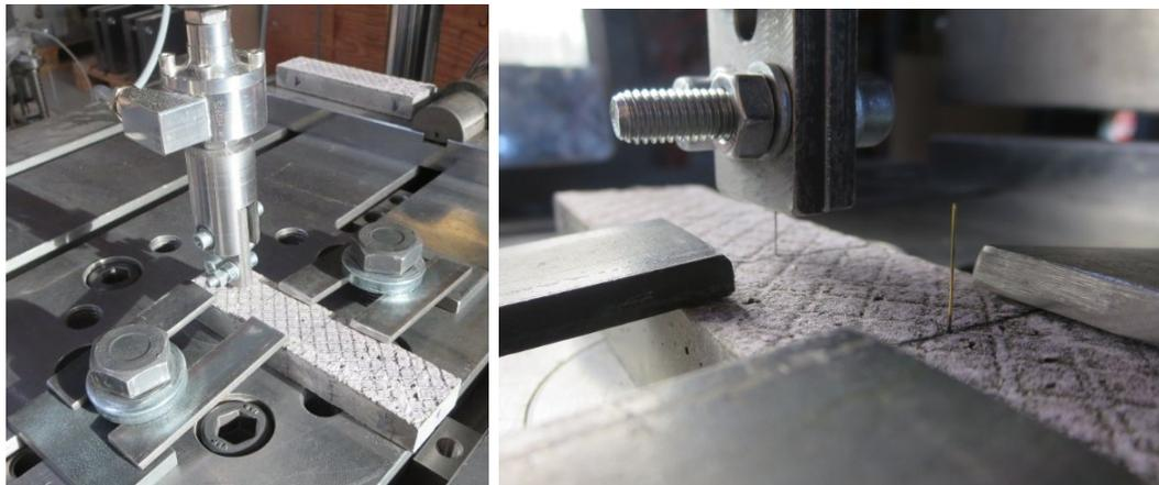
FIGURE 6.5.: Configuration of the single fibre pullout test. The embedded length equals a half length of fibre.
