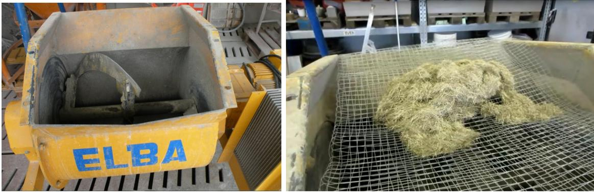
FIGURE 6.3.: Compulsory Mixer for preparation of UHPFRC.
