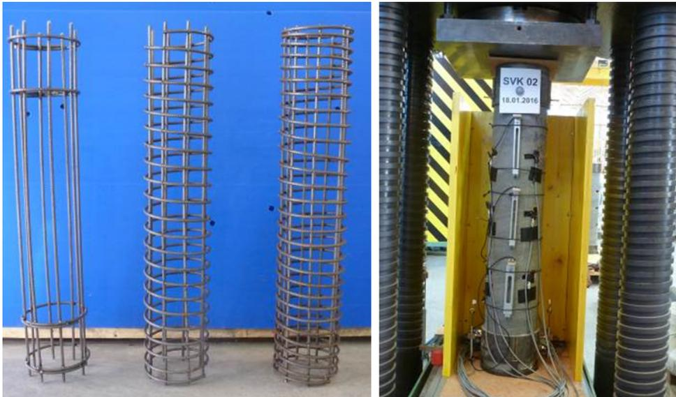
FIGURE 7.5.: Different amount of spiral reinforcement (Types A and C) and test setups for the UHPC columns.
