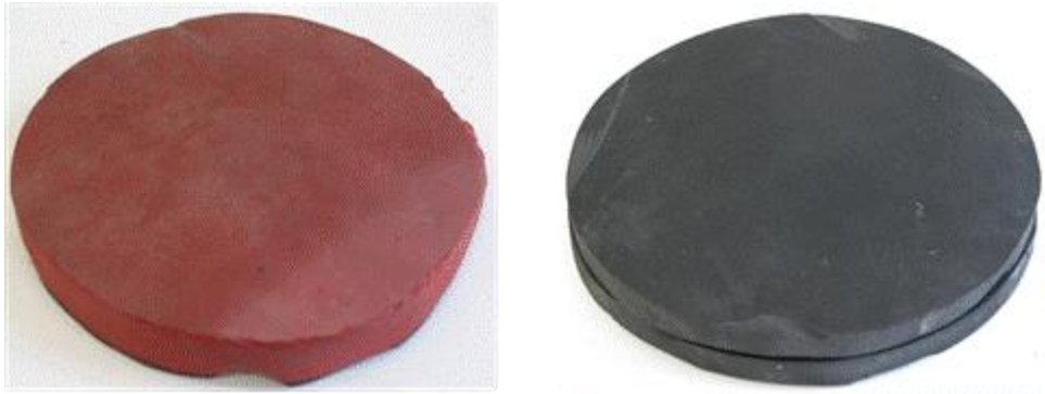
Figure 3-5: Rubber plates (red: soft; black: medium).
