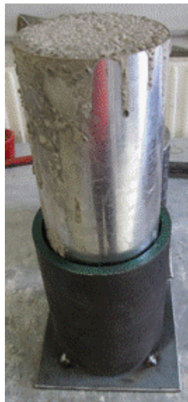
Figure 4-9: Bottom steel pipe and filling with lost formwork of test number (1.10).
