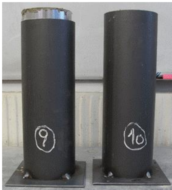
Figure 4-15: Yielding elements (test number (4.1) and (4.2)) of the fourth test series.
