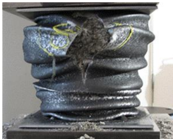
Figure 4-14: Stovepipe element with crack.
