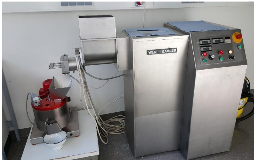
Figure 20: Extruder Pharmex T35, Gabler Maschinenbau GmbH, Lübeck, Germany
