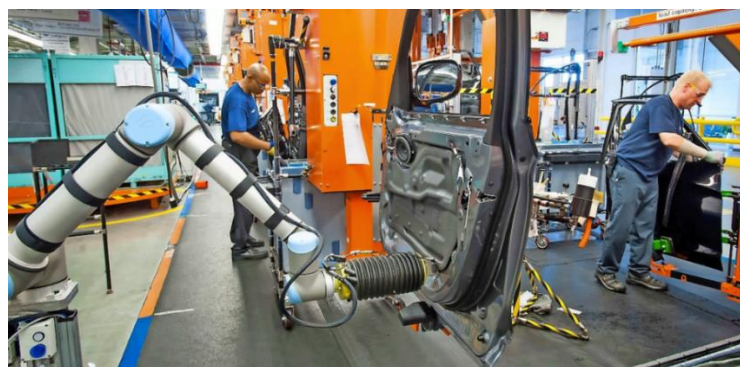
Figure 2-19 Co-working robot at line at BMW plant 106
